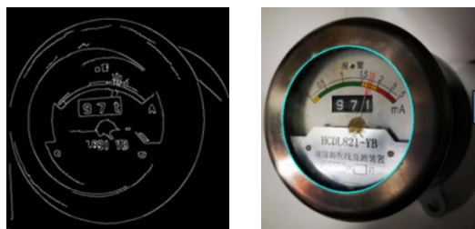
(a) Edge Detection Results (b) Inner Contour Fitting Results
