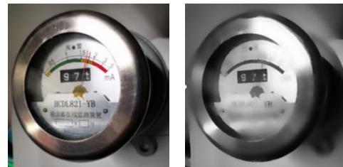
(a) Hough Transform Localization Result (b) Gaussian Denoising Result
