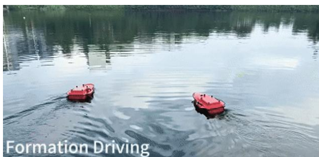
Figure 1. Formation cruising process of the USV swarm
