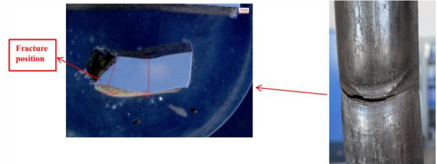
Figure 11. The macroscopic picture shows obvious deformation and the wall thickness at the breaking point is reduced 6.8X
